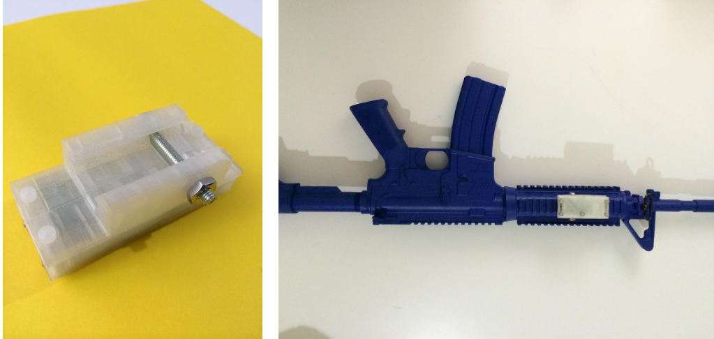
Fig 6: (left) the custom enclosure for the TI SensorTag (right) the enclosure mounted on the Picatinny rail of a rifle (standard M4 “style” Carbine used by most infantry type soldier).
