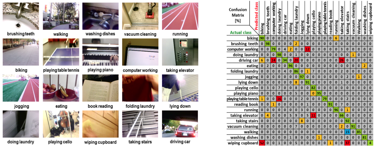
Fig. 1. (left) Snapshots from 20 daily activities of an individual. (right) Confusion matrix of activity decoding from head-mounted inertial data. Overall accuracy was 80.3% (Windau & Itti, 2013).
